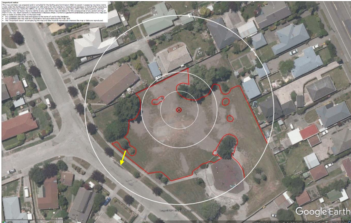
Figure 36: Absence of ejecta at the site for Dec-11 EQ. (The yellow arrow is pointing to the only place with fresh ejecta.)
