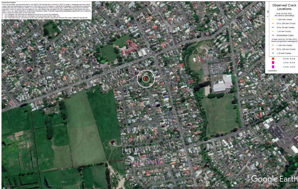
Figure 22: Absence of ground cracks indicating no lateral spreading for Canterbury Earthquake Sequence.
